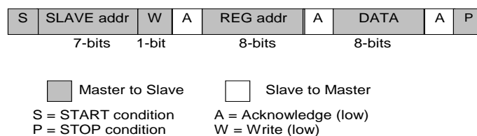
Figure 27: I 2 C Byte Write (SDA signal)
