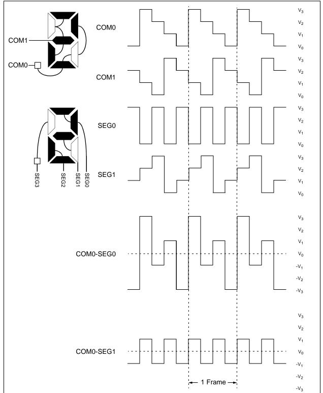
FIGURE 3: WAVEFORMS IN 1/2 MUX, 1/3 BIAS DRIVE
