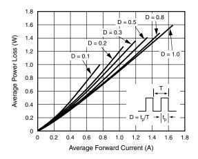
Fig. 2 - Forward Power Loss Characteristics
