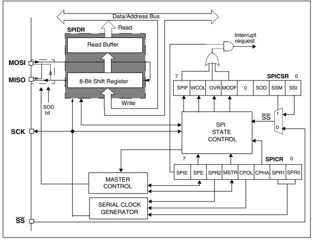
Figure 73. Serial peripheral interface block diagram
