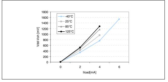
Figure 119. Typical  $V_{DD}$ - $V_{OH}$  vs.  $I_{IO}$  at  $V_{DD}$  = 5 V (standard)
