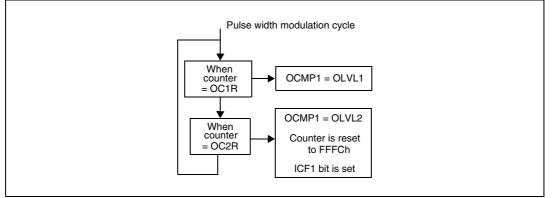
If OLVL = 1 and OLVL2 = 0 the length of the positive pulse is the difference between the OC2R and OC1R registers.
