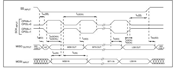
Figure 96. SPI slave timing diagram with CPHA=1
