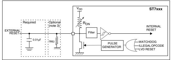
Figure 122. RESET pin protection when LVD is enabled
