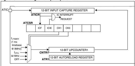
Figure 45. Block diagram of input capture mode
