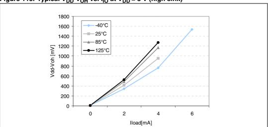
Figure 115. Typical  $V_{DD}$ - $V_{OH}$  vs.  $I_{IO}$  at  $V_{DD}$  = 3 V (high sink)
