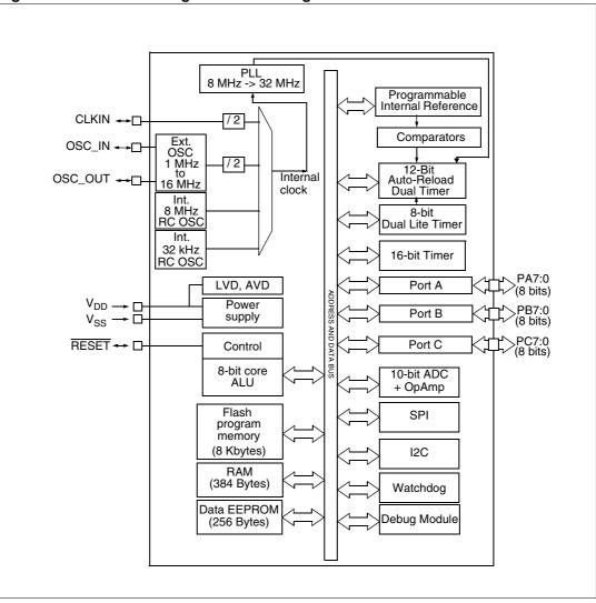
Figure 1. ST7LITE49K2 general block diagram
