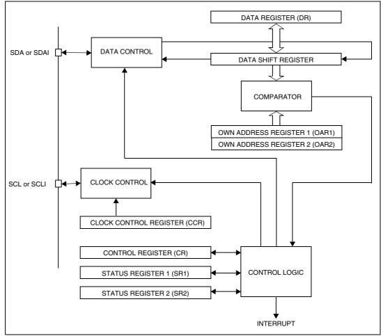
Figure 70. I<sup>2</sup>C interface block diagram
