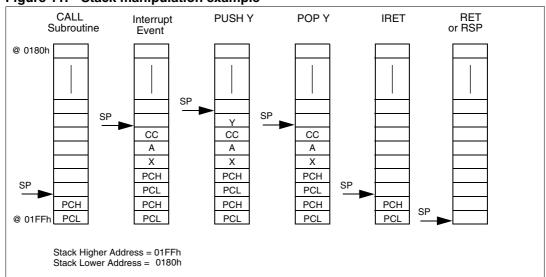
Figure 11. Stack manipulation example
