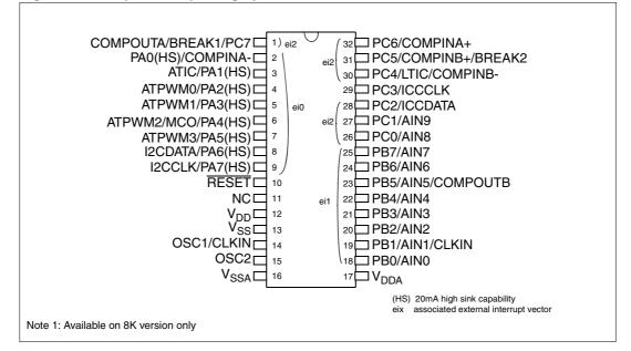
Figure 3. 32-pin LQFP 7x7 package pinout
