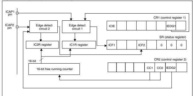
Figure 60. Input capture block diagram
