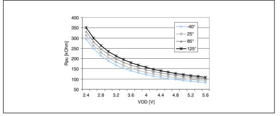
Figure 102. I<sub>pu</sub> current versus voltage at four different temperatures
