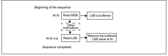
The user must read the MSB first, then the LSB value is buffered automatically.
