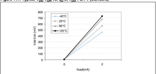
Figure 117. Typical  $V_{DD}$ - $V_{OH}$  vs.  $I_{IO}$  at  $V_{DD}$  = 2.4 V (standard)
