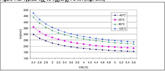
Figure 112. Typical  $V_{OL}$  vs  $V_{DD}$  at <sub>IO</sub> = 8 mA (high sink)
