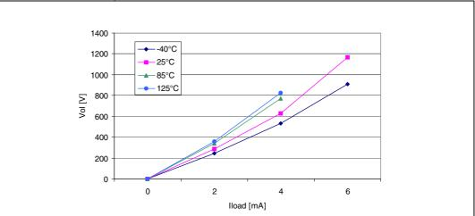
Figure 105. Typical  $V_{OL}$  at  $V_{DD}$  = 5 V (standard)
