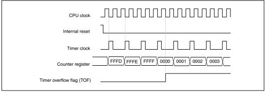
Figure 58. Counter timing diagram, internal clock divided by 4
