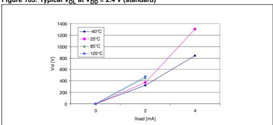
Figure 103. Typical  $V_{OL}$  at  $V_{DD}$  = 2.4 V (standard)
