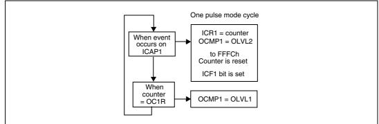
When a valid event occurs on the ICAP1 pin, the counter value is loaded in the ICR1 register. The counter is then initialized to FFFCh, the OLVL2 bit is output on the OCMP1 pin and the ICF1 bit is set.
