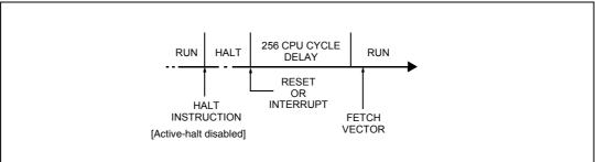
1. A reset pulse of at least 42 µs must be applied when exiting from Halt mode.
