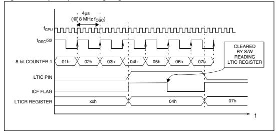
Figure 54. Input capture timing diagram
