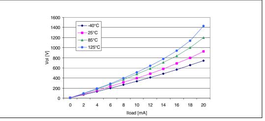
Figure 108. Typical  $V_{OL}$  at  $V_{DD}$  = 5 V (high sink)
