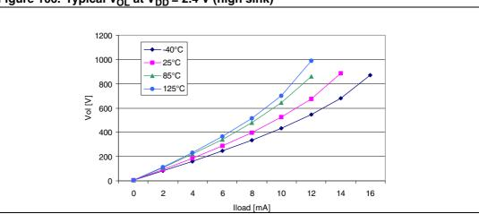
Figure 106. Typical  $V_{OL}$  at  $V_{DD}$  = 2.4 V (high sink)
