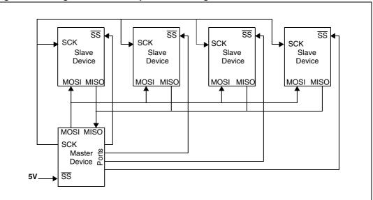
Figure 79. Single master / multiple slave configuration
