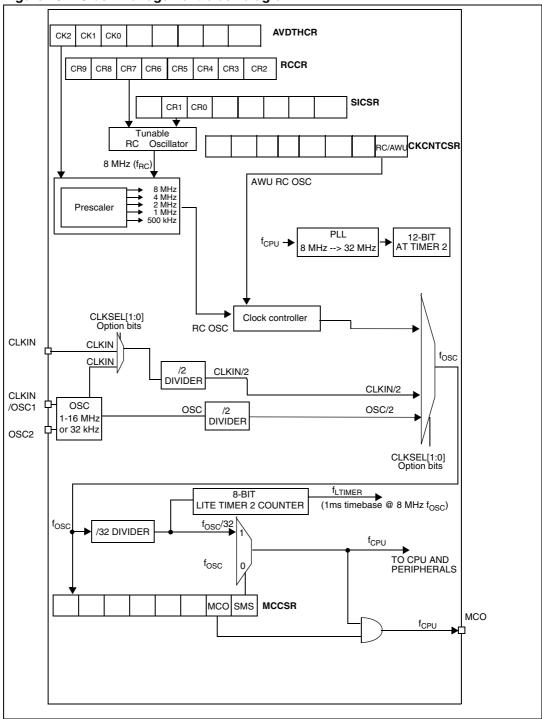
Figure 13. Clock management block diagram
