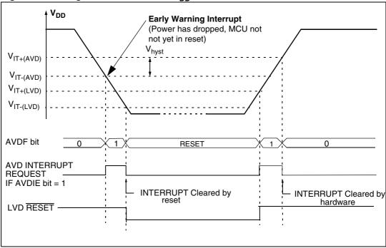
Figure 19. Using the AVD to monitor  $V_{DD}$
