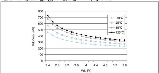
Figure 120. Typical  $V_{DD}$ - $V_{OH}$  vs.  $V_{DD}$  at  $I_{IO}$  = 2 mA (high sink)
