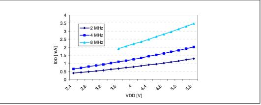
Figure 92. Typical  $I_{DD}$  in Slow mode vs.  $f_{CPU}$
