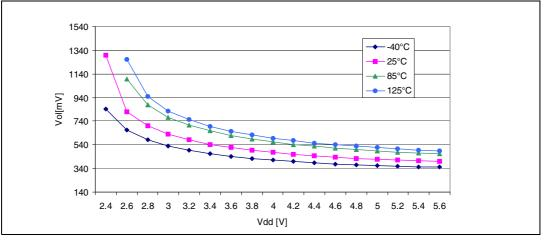
Figure 111. Typical  $V_{OL}$  vs  $V_{DD}$  at  $I_{IO}$  = 2 mA (high sink)
