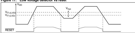
Figure 17. Low voltage detector vs reset
