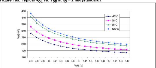
Figure 109. Typical V<sub>OL</sub> vs. V<sub>DD</sub> at  $I_{IO}$  = 2 mA (standard)
