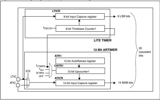
Figure 47. Long range input capture block diagram
