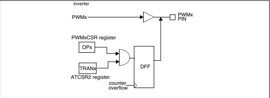
The Data Flip Flop (DFF) applies the polarity inversion when triggered by the counter overflow input.
