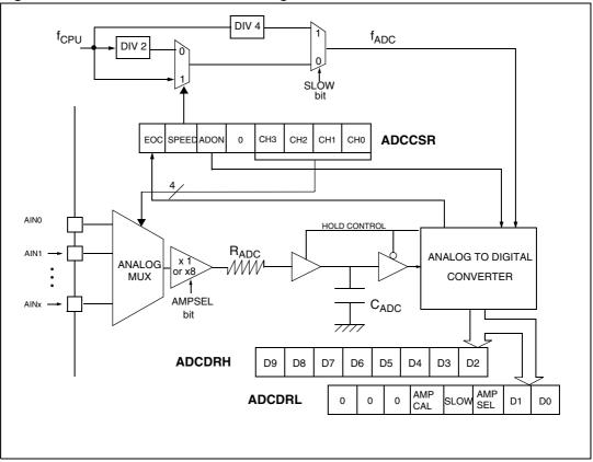
Figure 80. ST7LITE49K2 ADC block diagram
