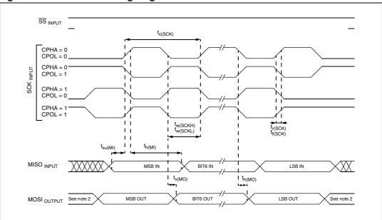
Figure 97. SPI master timing diagram
