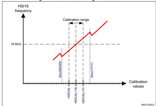
Figure 1. HSI oscillator trimming characteristics
