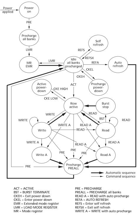
Note: This diagram represents operations within a single bank only and does not capture concurrent operations in other banks.
