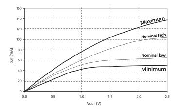
Figure 12: Full Drive Pull-Up Characteristics
