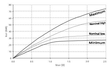
Figure 14: Reduced Drive Pull-Up Characteristics
