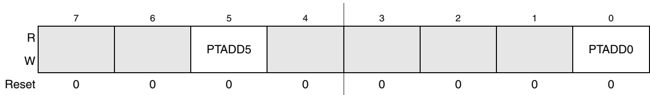
Figure 6-3. Data Direction for Port A Register (PTADD)
