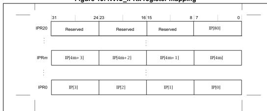
Figure 19. NVIC\_IPRx register mapping
