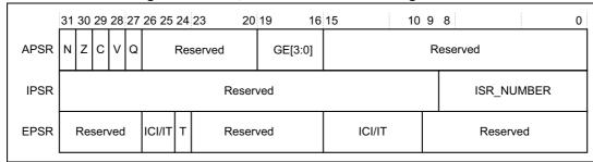
Figure 4. PSR bit assignments
