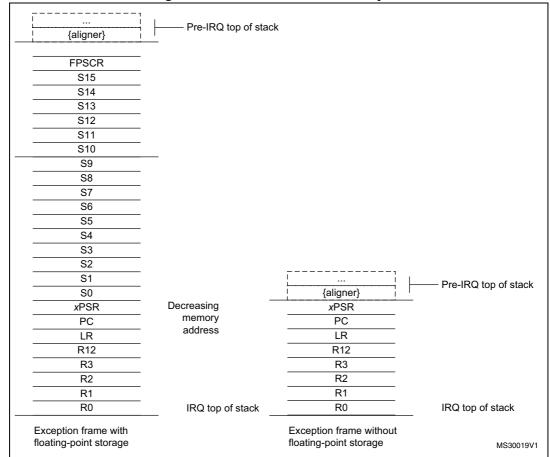
Figure 12. Cortex-M4 stack frame layout
