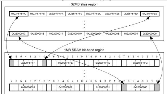
Figure 9. Bit-band mapping
