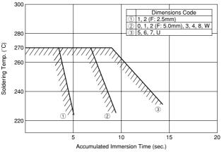
Perform soldering within tolerance range (shaded portion).
